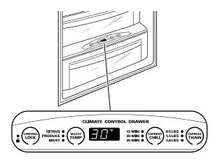
The Climate Control Drawer compartment is sealed to reduce the effect that the drawer temperature has on the rest of the refrigerator. When the drawer features are not being used, the temperature inside the drawer will be the same as the fresh food compartment.
