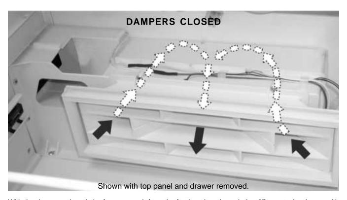
With the dampers closed, the fan moves air from the fan housing, through the diffuser, to the drawer. Air returns from the drawer, through the diffuser, to the fan compartment.
