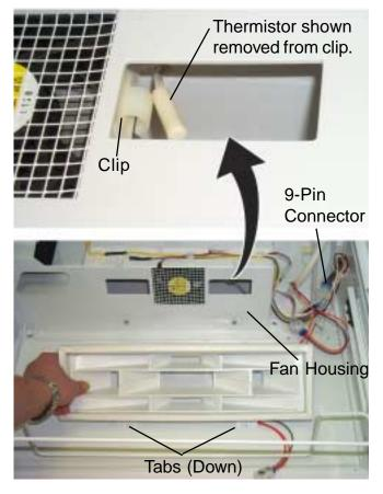
**Note:** All thermistors can be checked using Diagnostic Mode.
