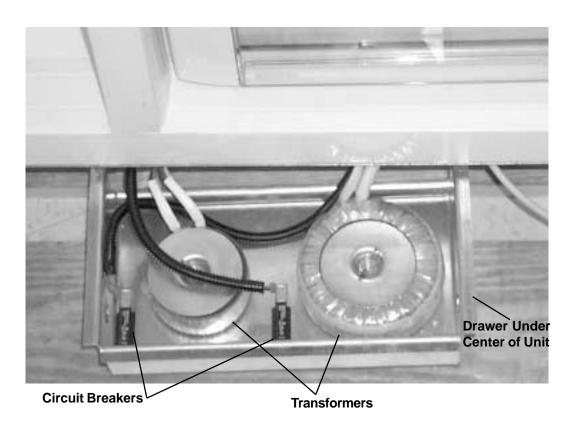
Figure 5 - Light Circuit Transformers
