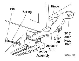
3. Remove 2 screws and the roller assembly from the rail. Replace roller if excessively worn.
