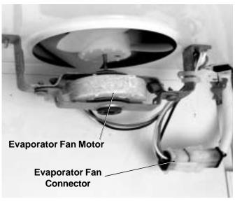
Figure 4 - Evaporator Fan
