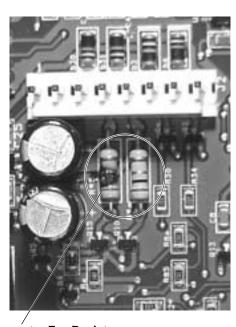
**Bad Evaporator Fan Resistor**
