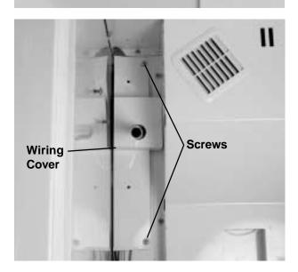
6. Remove 6 screws and evaporator fan cover.
