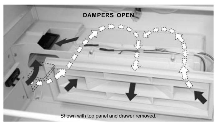
With the dampers open, cold air moves from the FZ compartment through the lower damper and into the fan housing. The fan blows the cold air through the diffuser into the drawer. The air returns from the drawer through the diffuser and into the fan housing. Air also moves over the top of the drawer, into the Climate Control Drawer compartment (not into the FF compartment), and then out of the compartment via the top damper.
