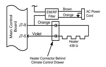
Heater resistance should be  $438\Omega$  and can be checked at 2 places:
