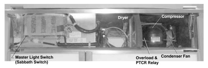
Figure 1 - Machine Compartment
