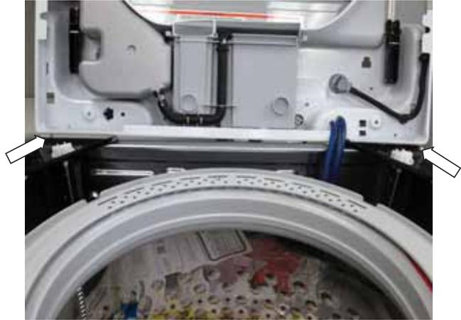
6. Using the backsplash screws, push the screws through the existing holes in the rear of the top cover.
