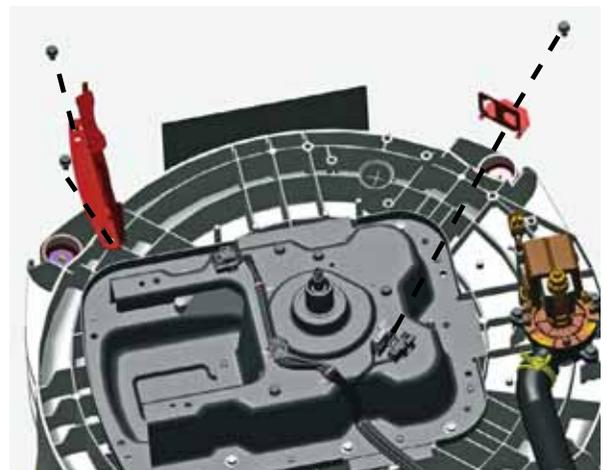
6. Remove the eight 3/8 hex bolts securing the platform to the bottom of the tub.
