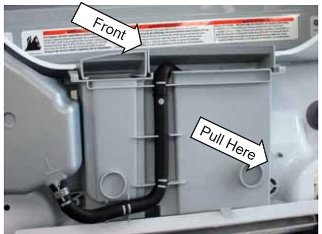
7. When the dispenser box is reinstalled, the front of the box needs to be inserted first.
