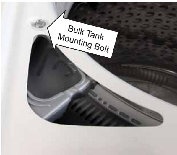
2. Pry the tabs of the bulk tank out from under the lip of the top cover. Again, be careful not to pry too hard against the top cover lip. It can be bent.
