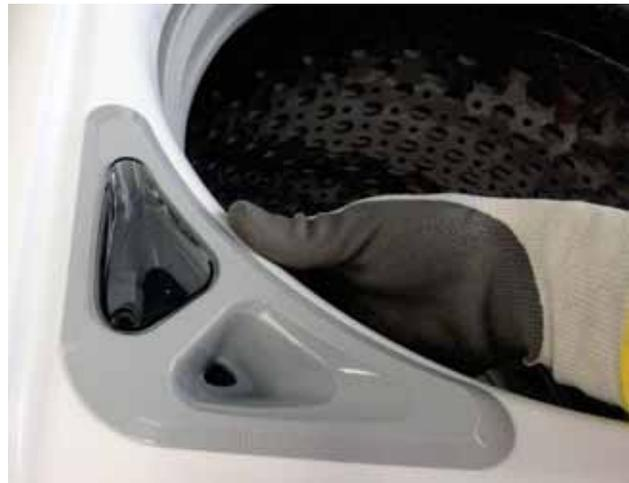
2. Removing the funnel gives access to the bulk tanks 3/8 in. mounting bolt.
