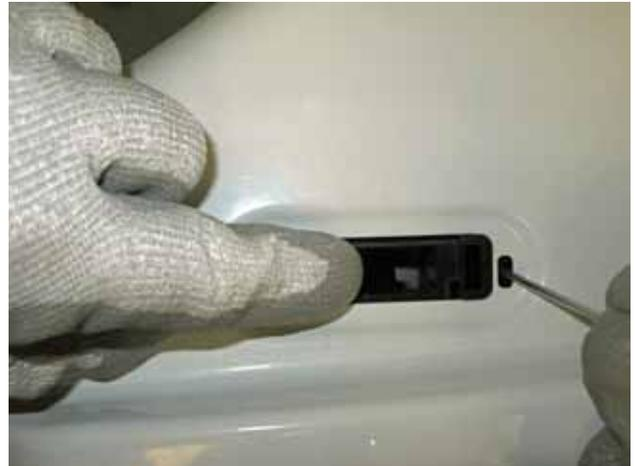
3. Slide the lock assembly to the left first to disengage the right lock body tab. Then slide to the right, allowing the lock assembly to disengage from the top cover.
