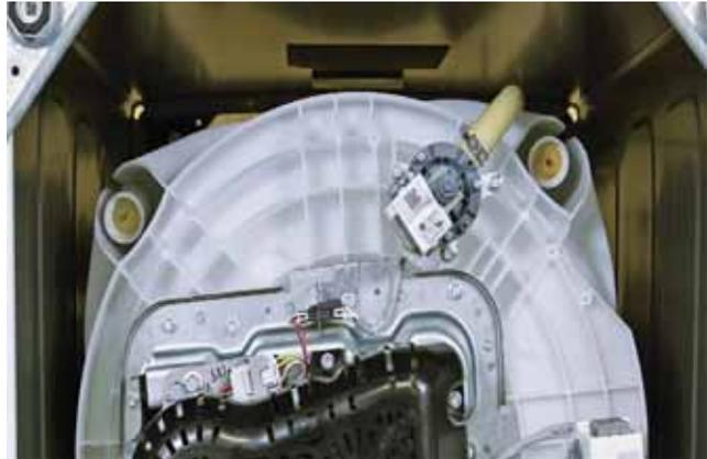
5. Remove three 3/8 hex head bolts securing the pump to the tub.
