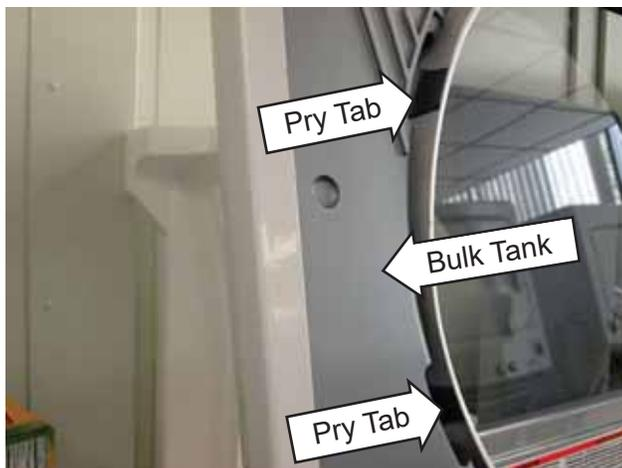
3. Lift the bulk tank out from the top cover.
