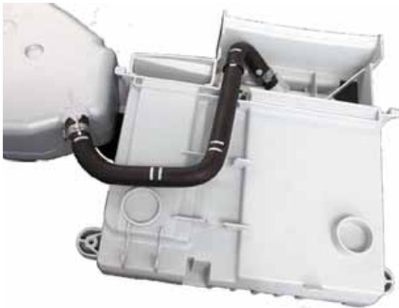
3. Unclip the dispensing tube from the mounting bracket.
