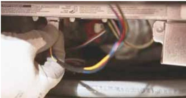
4. Release the wire clip holding the harness to the tub. Push up on the wire harness to release the harness.
