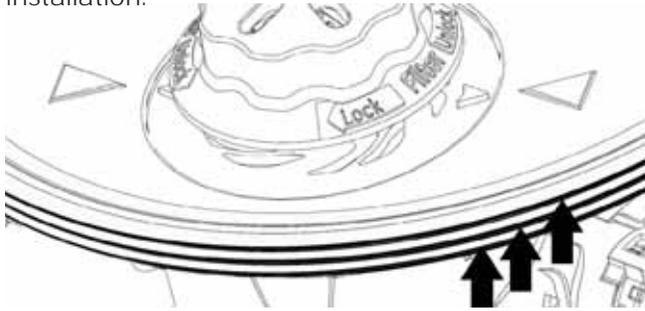
**Single Use Clamp Removal Tip:** Use a small screwdriver inserted into the ear of the clamp and move the handle back and forth to loosen the clamp. The clamp can be removed and discarded when the component is removed.
