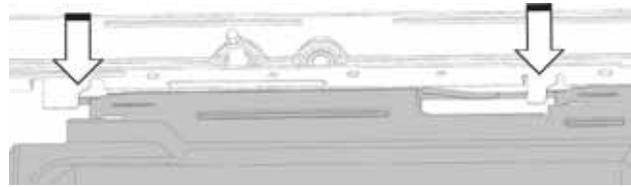
3. Slide the pan to the back of the dishwasher to engage the tabs and lock the pan in place.
