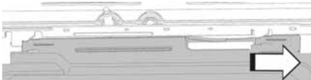
4. The pan will drop to the floor and can be removed from under the dishwasher.
