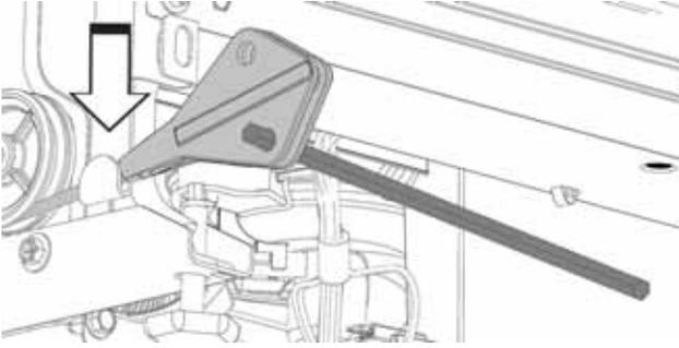
**Caution:** If the cable is released before it is secured in the clip, the spring and cable may become disconnected. Depending on the model and installation, reconnecting may require the dishwasher to be removed from the installation.
