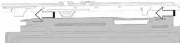
2. Lift the pan upward until it contacts the base rail tabs.
